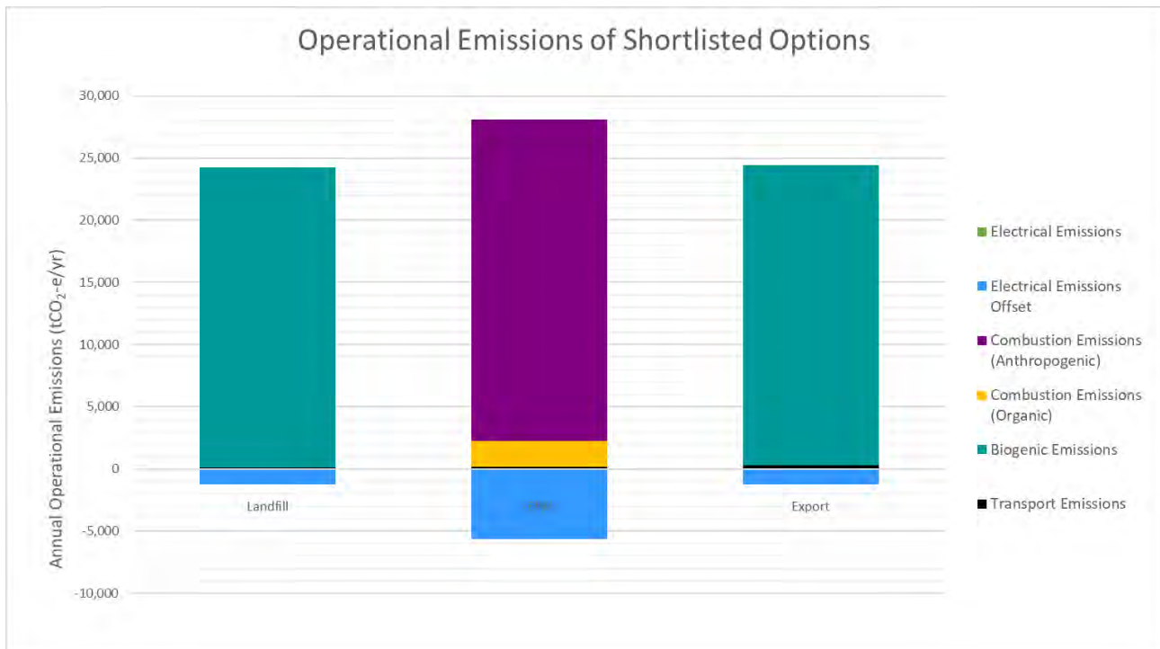
Figure 7: Summary of Gross Operational Emissions (including abated emissions from energy generation) by Source
